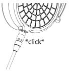
All Dan Clark Audio planar-magnetic products use Hirose-style connectors. To attach your cable hold the male connector by the boot and rotate it into the female receptacle on the headphone until you feel it click into place. To release the cable pull down on the top of the connector's metal jacket.
