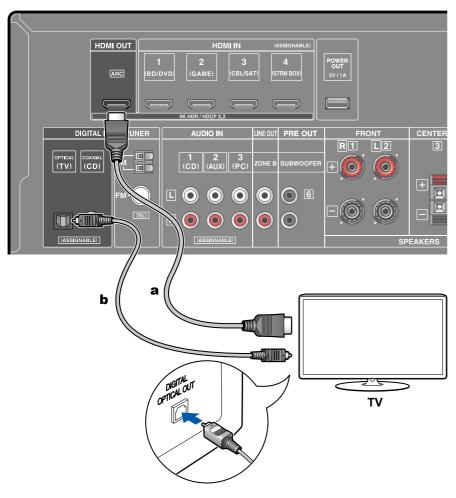
If the TV does not support the ARC (Audio Return Channel) function (\*), connect an HDMI cable and digital optical cable.
