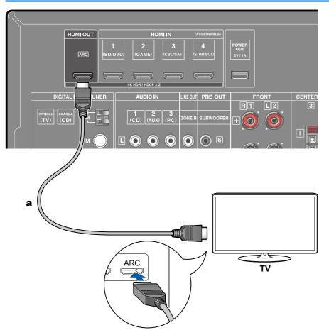
If the TV supports the ARC (Audio Return Channel) function (\*), use only the HDMI cable to connect with the TV. Use the ARC-compatible HDMI IN jack of the TV for connection. You connect the HDMI cable to the port labeled OUT on the receiver side.
