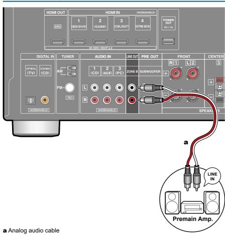
While performing playback in the main room (ZONE A), you can enjoy 2-ch audio of the same source in the separate room (ZONE B) at the same time. Use an analog cable to connect the ZONE B LINE OUT jack of this unit and the LINE IN jack of the pre-main amplifier in the separate room.
