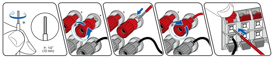
Make correct connection between the unit's jacks and speaker's jacks (+ side to + side, and - side to - side) for each channel. If the connection is wrong, a bass sound will not be reproduced properly due to reverse phase. Twist the wires exposed from the tip of the speaker cable so that the wires do not stick out of the speaker terminal when connecting. If the exposed wires touch the rear panel, or the + side and - side wires touch each other, a malfunction may occur.
