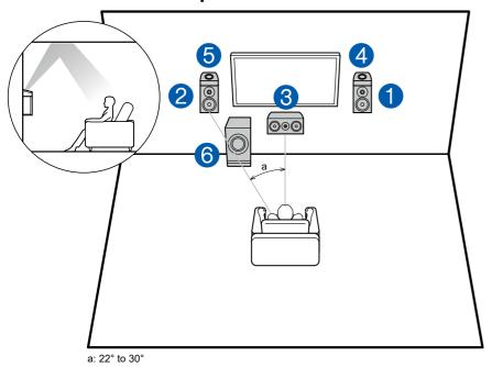
This is a 3.1-channel system consisting of front speakers, a center speaker, and a powered subwoofer, with the addition of Dolby enabled speakers (front), a type of height speaker. Dolby enabled speakers are special speakers designed to face the ceiling, so that the sound is heard from overhead by bouncing the sound off the ceiling. Installing the height speakers will enrich the sound field feeling in the upper space.
