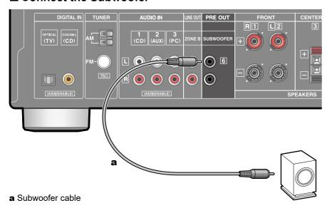
Connect a powered subwoofer with this unit using a subwoofer cable. Up to two powered subwoofers can be connected. The same signal is output from each SUBWOOFER PRE OUT jack.
